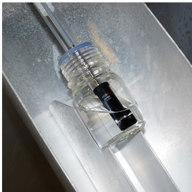
Fig. 2: Acid analysis set-up with all-quartz transmission probe and sample.
