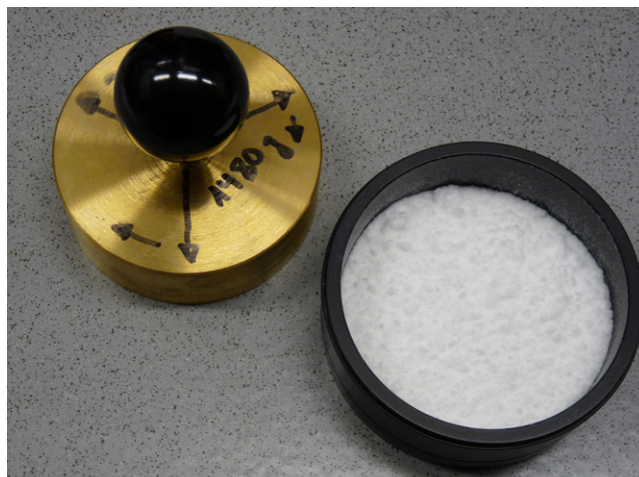
Fig. 7: Sample preparation: approx. 10 g of dried NC is filled into the BUCHI NIRFlex-Solids-Cell; the NC is then compressed by inserting a plunger (approx. 1.5 kg).
