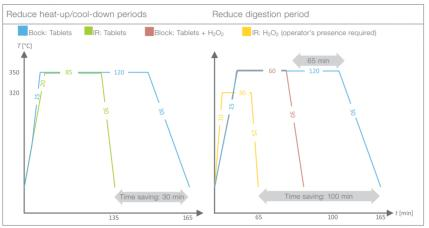
Use optimized «Kjeldahl Throughput» solution to get the highest sample throughput (batch size: 20 samples)
