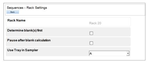
"Determine blank(s) first": Blanks are determined first, followed by sample measurements.
