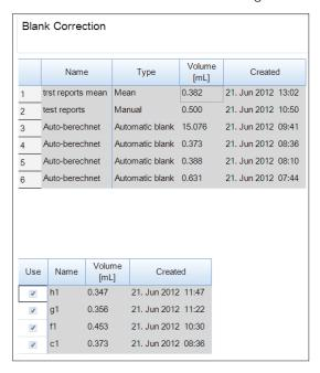
When a row is selected, the corresponding measured blank(s) is/are displayed in the lower table. If a blank is identified as outlier or should not be included in the result calculation, it can be removed by selecting the checkbox. An auto-calculated blank, that has been modified, is marked with an asterisk (\*).
