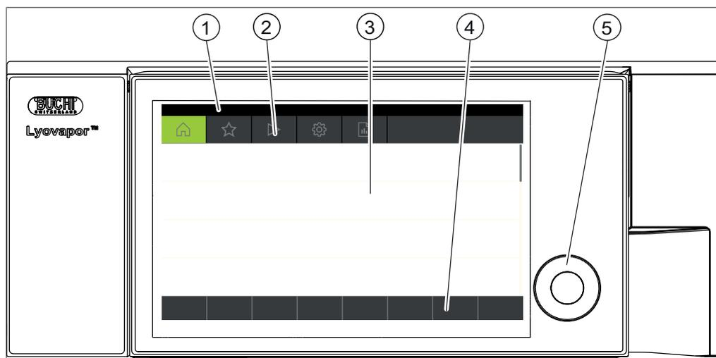
Fig. 17: Layout of Pro control panel
