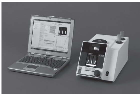
Fig. 5.1: Connection of Melting Point M-565 with the MeltingPoint Monitor software.
