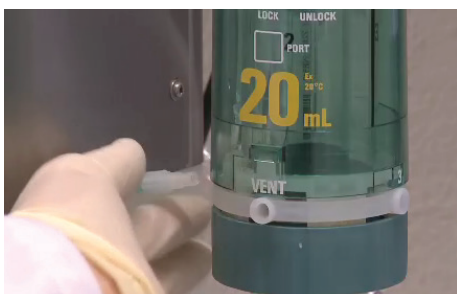
Fig. 5.8: Connection of the FEP hose at the dosing unit
