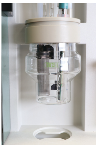
Fig. 5.17: Colorimetric titration setup
