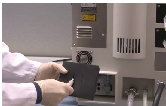
Fig. 5.10: Guidance of the cable through the cut-out
