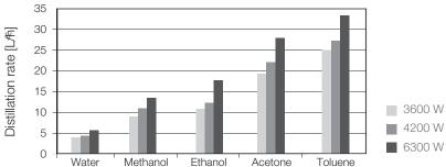
The maximum achievable distillation rate is not just related to the heating capacity, but also on rotation speed, flask size and temperature difference between bath and cooling.
