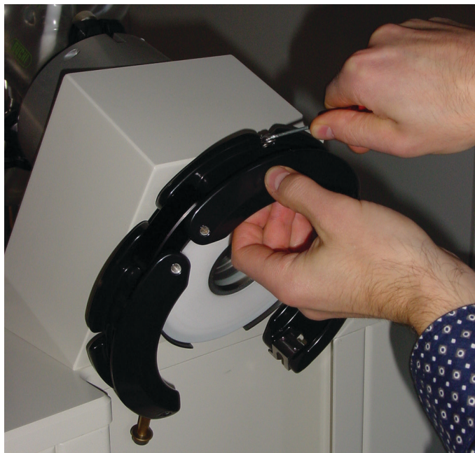
Fig. 6.1: Taking apart the snap flange coupling
