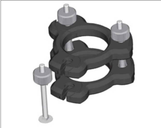
Fig. 4.2: Attachment of the EasyClamp
