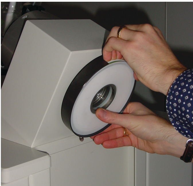
Fig. 6.3: Removing the evaporating flask seal
