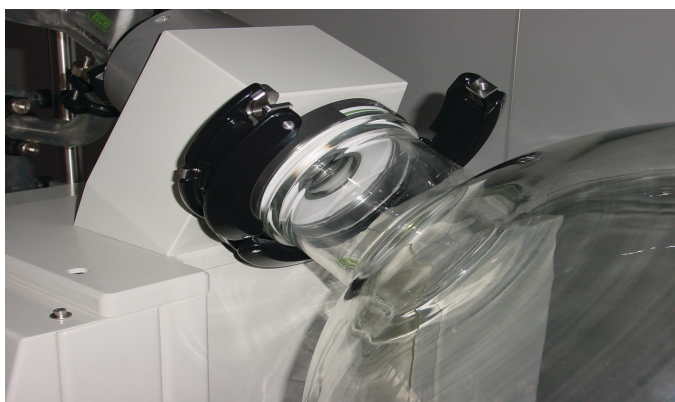
Fig. 4.8: Fitting the flask
