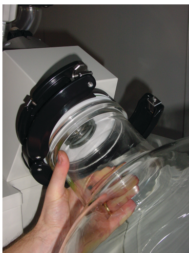
Fig. 4.13: Removing the flask
