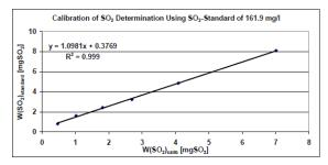
**Figure 7:** Calibration curve for the determination of total  $SO_2$  and the linear equation correlating the measured  $SO_2$  amounts (x-axis) to the theoretical  $SO_2$  contents (y-axis).
