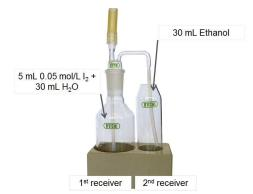
Figure 4: SO2 absorption vessel
