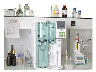
Figure 1: Setup for SO2 determination
