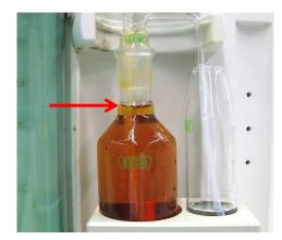
Figure 5: 1st receiver filled with destillat to the bottle neck
