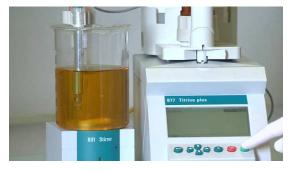
Figure 6: Titration setup with Pt-electrode
