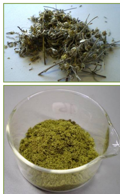
Figure 1: Plant material (Genépi) before and after homogenization (ultra centrifugal mill, 1 mm sieve)
