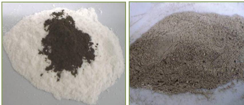
Figure 3: Dried sewage sludge with Celite (left) and sample mixed Celite (right)
