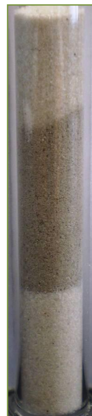
Figure 4: Ottawa sand bed, with the sample and another sand bed on top
