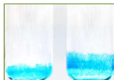
Figure 16: 0.2 g hydrocarbon grease evaporated at 170 rpm (left) and at 300 rpm (right).
