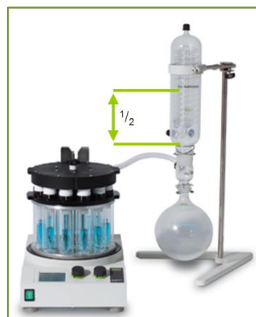
Figure 17: The vacuum and cooling conditions are ideal when the condensate covers approximately half of the height of the condenser.
